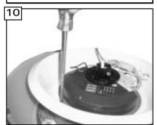
Install 4 screws to hold reflector in place.
